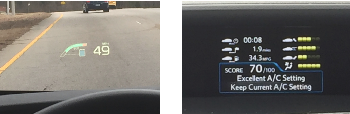
Figure 8 The Prius HUD allows drivers to see how their driving impacts the car's eco-friendly status and delivering a brief message at the end of every driving session.
