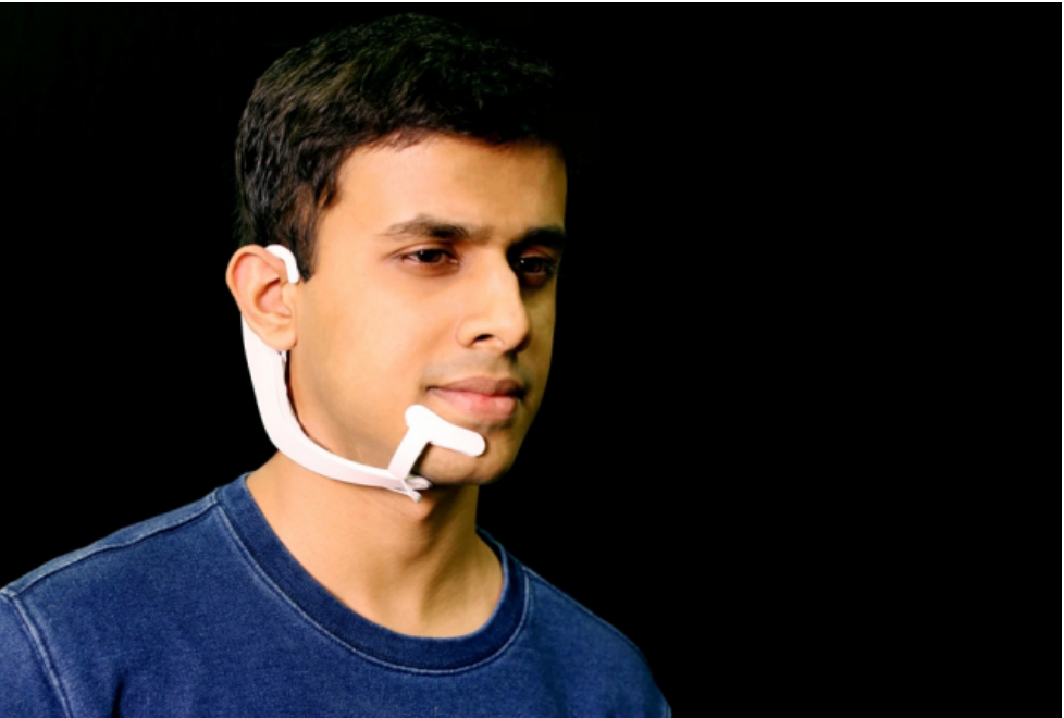
Figure 34 AlterEgo: AlterEgo is a non-invasive, wearable, peripheral neural interface that allows humans to converse in natural language with machines, artificial intelligence assistants, services, and other people without any voice—without opening their mouth, and without externally observable movements—simply by articulating words internally.
