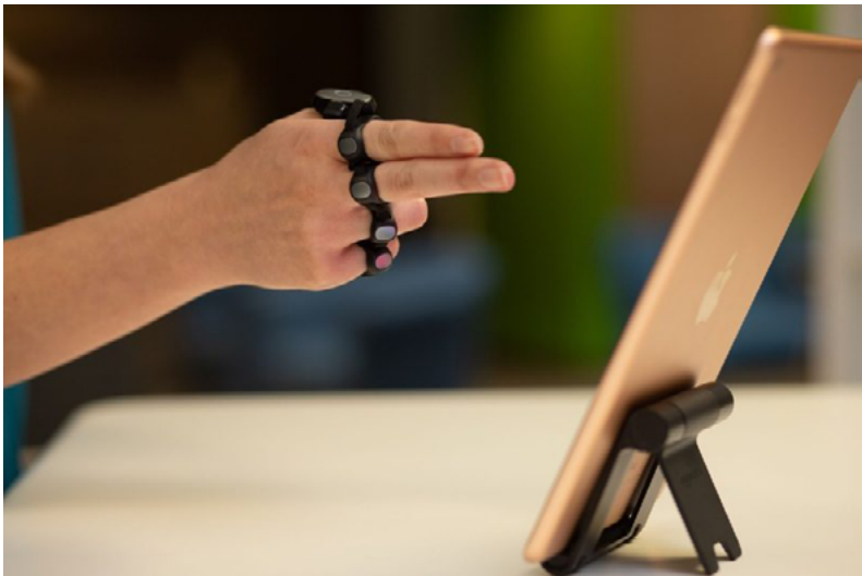
Figure 31 Tap Strap 2: It's an all in one, wearable keyboard, mouse & air gesture controller.
