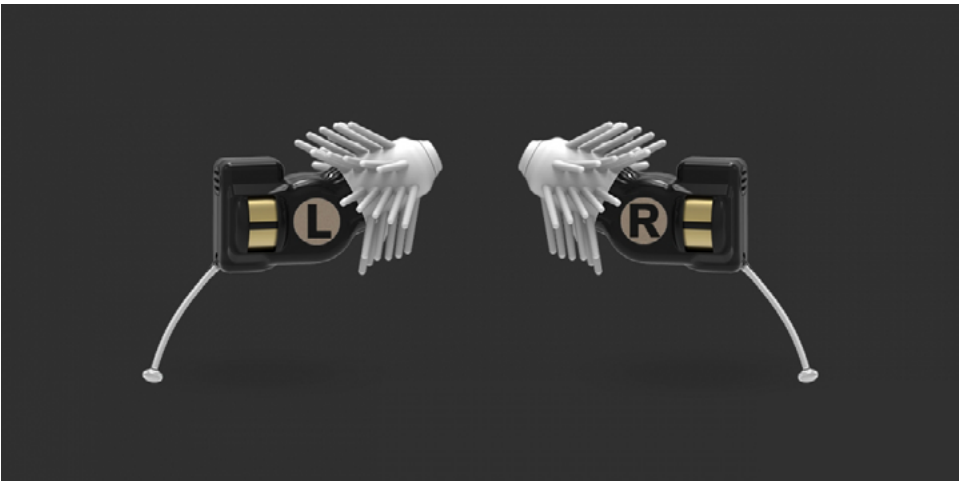
Figure 26 Eargo: Eargos amplify speech while reducing background noise, making it easier and more comfortable to hear in noisy settings.
