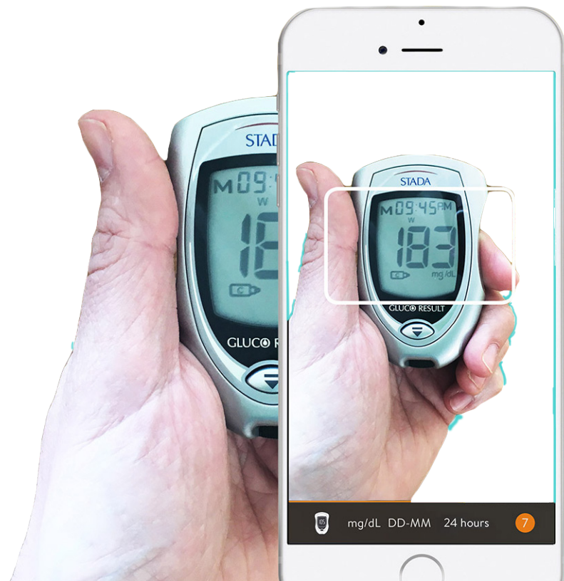
Fig. 11 MySugr is a mobile application that can sync data from blood glucose monitors by scanning the screens of the monitor devices. This tool influenced my decision to integrate blood glucose level testing into TYPE2U and how that data influences the products for future food shopping trips ("MySugr.Com.").
