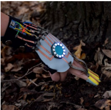
Figure 2.6.7 Hand-substrate interface measuring soil.
